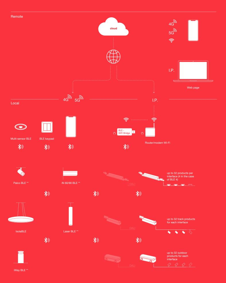
Max 320 DALI addresses x network / \*Bridge and WiFi are required for remote control from PC, smartphone, tablet and the scheduler / \*\*BLE products
