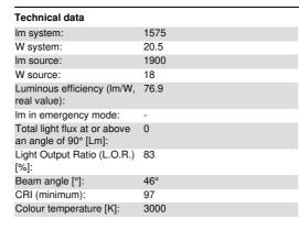
MacAdam Step: Life Time LED 1: > 50,000h - L90 - B10 (Ta 25°C) Lamp code: LFD Number of lamps for optical
