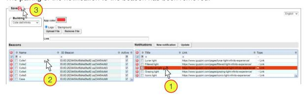
It is possible to pair several beacons to the same notification; this can be useful when you want to push the same notification in a large area, using several beacons and avoiding using only one beacon with high power.
