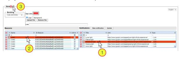
To cancel the pairing, select the notification (both the notification and the paired beacon will be displayed in red), click on the beacon (the beacon will no longer be red while the notification will remain red). In this condition, press 'Save' in the top left corner. A flashing 'Saved' information will be displayed for a few seconds after a successful operation.
