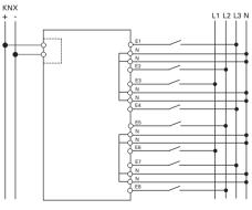
The N conductors must be connected to the device. Inputs E1 to E4 have a common potential (4 x N, top row) and inputs E5 to E8 have a common potential (4 x N, bottom row). Inputs E1 to E4 and E5 to E8 can be assigned to each other with different phases.
