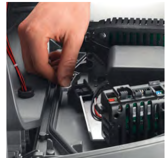
Tool-free replacement of power supply
