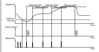
Where this differs from the presence detector is that the movement detector changes to non-brightness-dependent mode once the start of movement action (sending an ON telegram) has been carried out. Here freshly detected movements can retrigger the staircase timer. Unlike the presence detector, the movement detector cannot process the brightness jump and there is not even any setting of a hysteresis.
