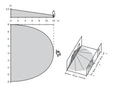
In order to ensure continuous monitoring, e.g. of a long hall, the areas of detection of the individual movement detectors have to intersect.
