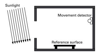
Optimal light conditions for actual value correction. Measurement results at the installation site or at the reference area are affected equally by natural light.
