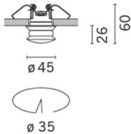
**Product code**BU07: Wall/ceiling recessed, ø45mm luminaire without an electronic transformer - Warm White - 360° radial effect **Attention! Code no longer in production****Technical description**
