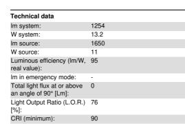
Colour temperature [K]: 3000 MacAdam Step: > 50,000h - L90 - B10 (Ta 25°C) Life Time LED 1: Lamp code: LED Number of lamps for optical 1 assembly: ZVEI Code: LFD Number of optical assemblies: Control: DALI-2
